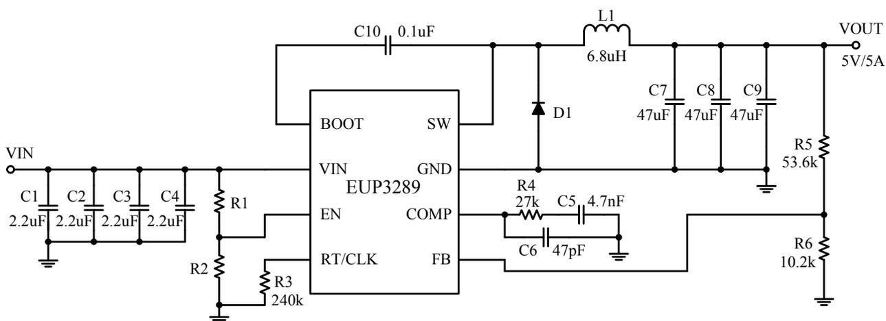
Figure 1. Application Circuit
